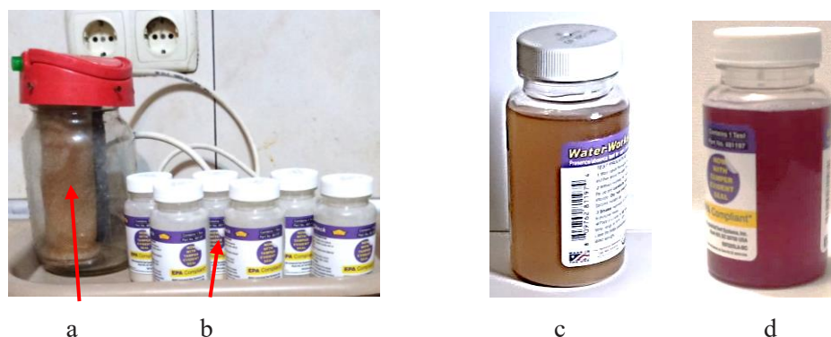
Fig. 3. Testing the presence of E. Coli bacteria in wastewater samples: a – the laboratory electrochemical water activator; b – WaterWorks™ Bacteria Check tests; c – the test of wastewater samples without anolyte disinfection (positive – living bacteria are present); d – the test of wastewater samples after disinfection with anolyte (negative – no living bacteria present)
